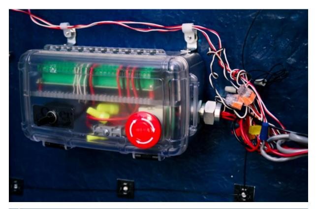
The image at the left shows the interface box with MaxDome II card mounted inside. The angle brackets at the top are used with stainless steel flat head screws to mount the box near the bottom of the rear shutter. A more sophisticated interface box with additional relays and a soft-start card for the motor (Chris Erickson, Summit Kinetics) will be installed in the future.
