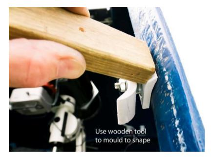
Here's how I solved the problem with the poorly fitting pulleys. The guides on the pulleys are PVC and will tolerate a bit of heating to reshape them. I used a hobby style heat gun to gently warm the PVC.
