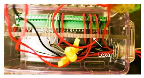
A piece of ¼ inch Lexan was cut to fit the inside of the box and serves as the mounting platform for the interface card. It is held in place with stainless steel screws on the sides and back.
