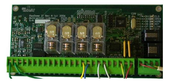
For control of the shutter I used the MaxDome II interface cared from Cyanogen. This is the same card used for controlling rotation of the dome, but configured to operate the shutter. It consists of a series of relays along with connections for open and closed switches, a manual operation switch, and a magnetic inductance antenna for communication with the rotation controller.
