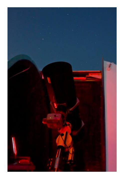
The automated shutter now allows unattended imaging. I use the ASCOM dome control panel, or the dome control routines incorporated into MaximDL to open and close the shutter, and to park the dome. The dome is routinely slaved to the mount.
