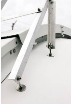
The 12VDC 5Ah sealed battery is supported by an aluminum frame which mounts on the inside of the rear shutter panel. All of the components are mounted using flat-headed stainless steel screws counter-sunk in the fiberglass dome to prevent any obstruction to the upper and front shutters as they open or close.
