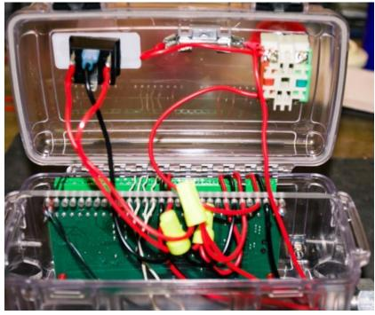
The hinged front of the box opens to allow easy access to the various connections. A series of 0.5 mm holes were drilled in the Lexan shelf to provide strain relief for the wires connected to the junction block of the MaxDome II card.
