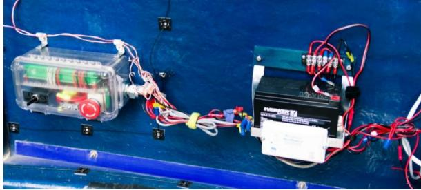
Here is the layout of the interface box and battery assembly mounted to the rear shutter. Mounting in this location prevents the box or battery from protruding excessively as the dome rotates.
