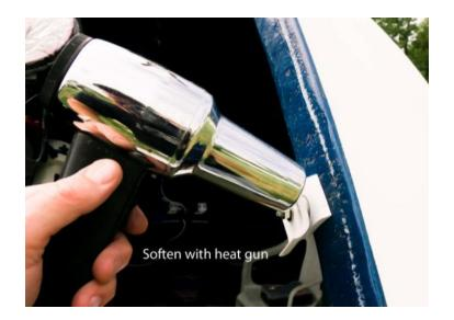
Then using a wood block I pressed the guide to match the shape of the shutter flange and held until the PVC cooled. If done carefully this makes each pulley have a custom fit and does not interfere with the movement of the pulley. The same technique can be used on the curved guides to form them to allow the shutter mechanisms to clear.
