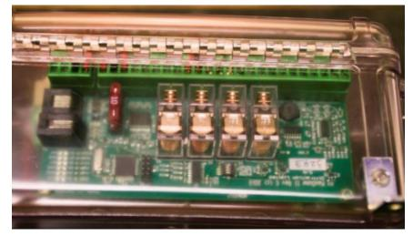
I mounted the MaxDome II card in an Otterbox 3500. This provides protection from the environment while allowing easy access to the various connections. Shown at the right is the front of the box with the manual control switch and an emergency KILL button that removes power to the interface card and shutter motor.
